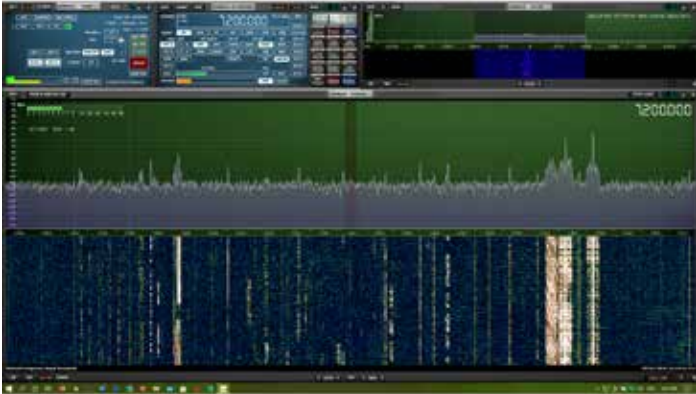
An SDR receiver on shortwave showing the signals of broadcasts and amateur radio signals
