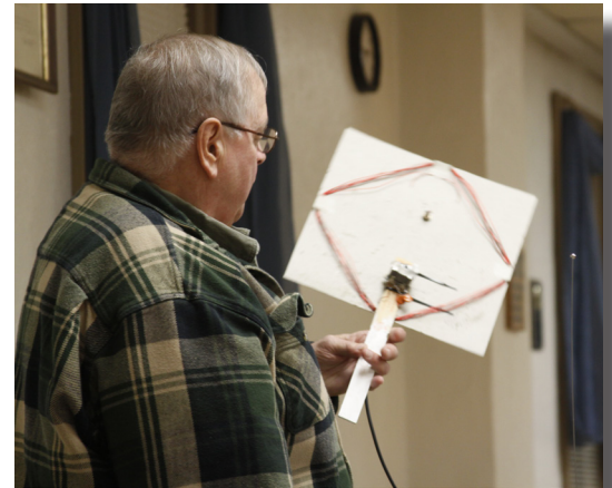
Steve demonstrating his simple receiving loop for tracking down noise in the shack
