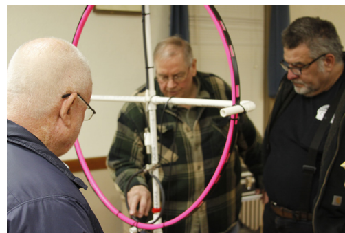
Steve shows his compact 40 meter loop transmitting antenna. Using it indoors he made contacts 600+ miles away Check out the pink hula hoop frame!
